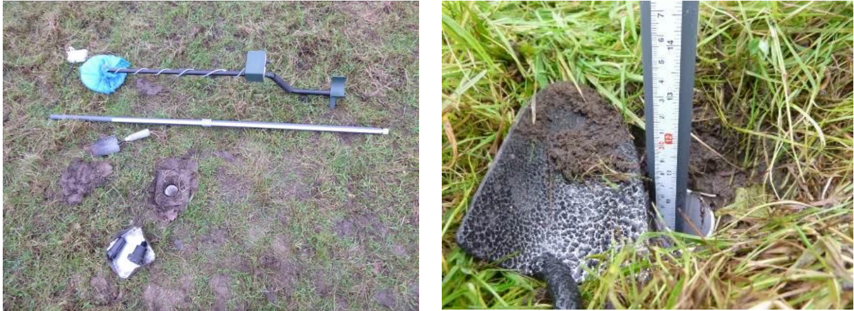
Figure 9. Dipwell reading equipment (metal detector, buzzing stick, trowel, screw cap and tread-plate)
