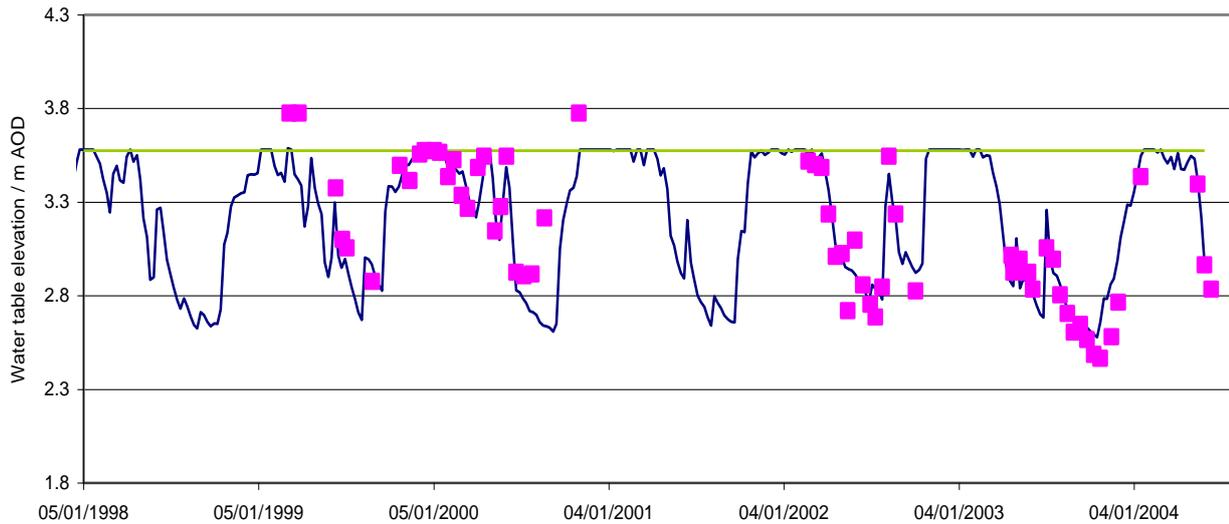
**Figure 1.** Model output (dark line) for a central tubewell at East Cottingwith compared to field observations for that well (square symbols). The ground surface elevation is shown by the horizontal line at 3.58 m AOD. (Note that the model does not predict depth of surface water).
