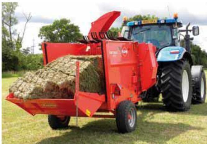
The bale is loaded into the rear of the spreader, chopped and then spread over the grassland through a funnel. The angle of the funnel and flow rate are adjustable, allowing the depth of the green-hay layer and the area of distribution to be altered. This method is quick and efficient. © Catherine Hosie
