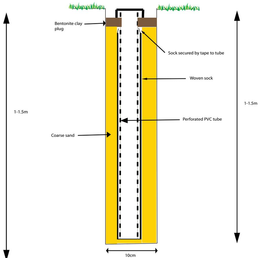
Note: the gap between the sock and surrounding hole should be filled with coarse sand to aid water movement into the dipwell
