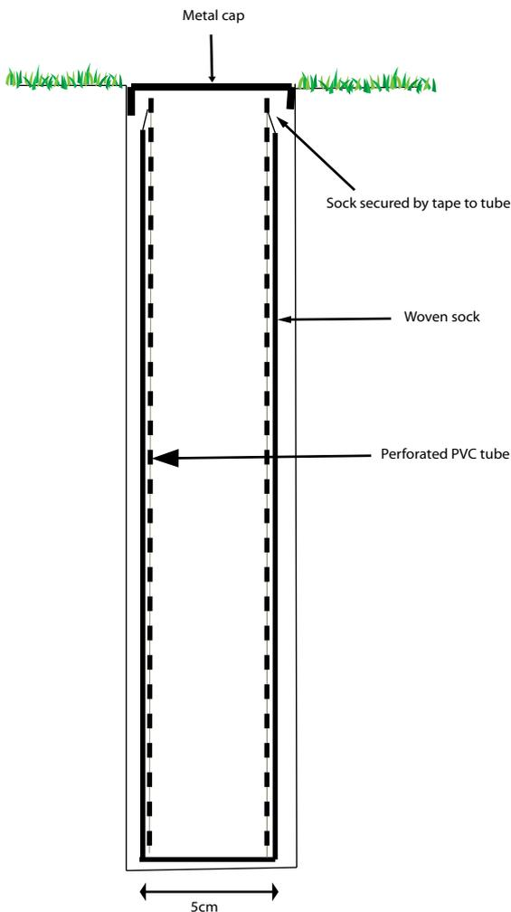
Figure 3. Dipwell in less permeable soil
