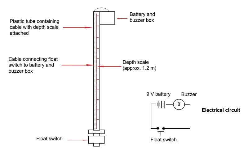
An alternative design would be to replace the plastic tube that carries the cable and holds the tape measure, with a simple tape measure and flexible cable. Attach the cable to the back of the tape measure, and attach the float switch and battery/buzzer box as described, and you have a buzzing tape measure that is easier to carry and make.
