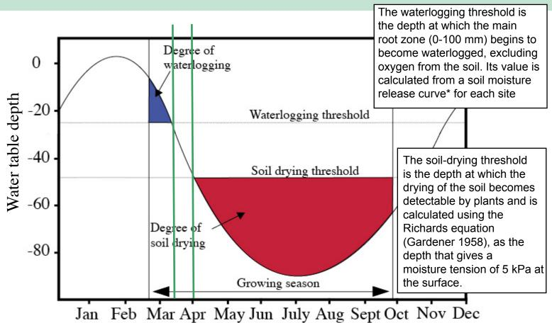
So during March in this example , the site demonstrates water-logging. The SEV is calculated from the area shaded blue.
