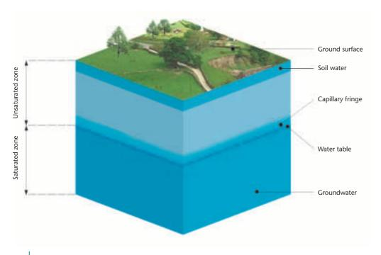
Figure 2 Profile of subsurface water With permission of the UK Groundwater Forum
