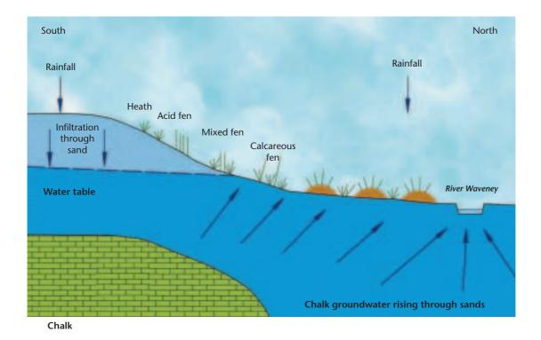
Figure 16 Section through Redgrave and Lopham Fen With permission of the UK Groundwater Forum
