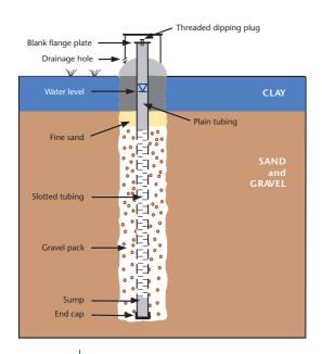
Figure 6 Monitoring borehole for confined conditions
