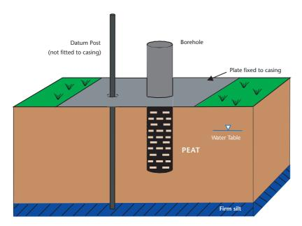
Figure 9 Setting a borehole datum post
