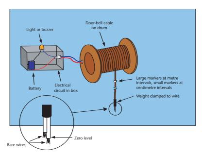
Figure 10 Home-made dip-meter With permission from 'Field Hydrology' by Rick Brassington
