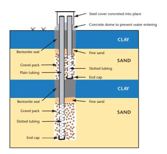
Figure 8 Nested piezometer
