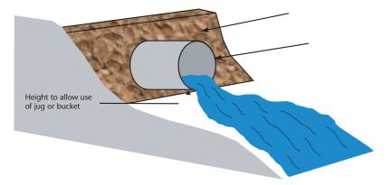
Figure 13 Measuring spring flow using a catch-pit With permission from 'Field Hydrology' by Rick Brassington
