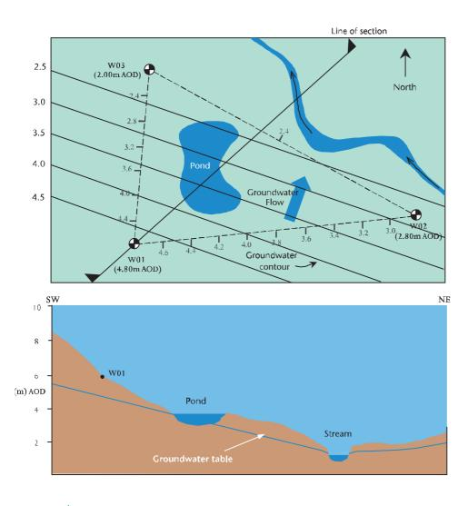
Figure 15 Groundwater contours and cross-section
