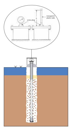
Figure 7 Monitoring set-up for artesian conditions
