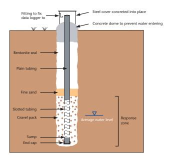
Figure 5 Monitoring borehole
