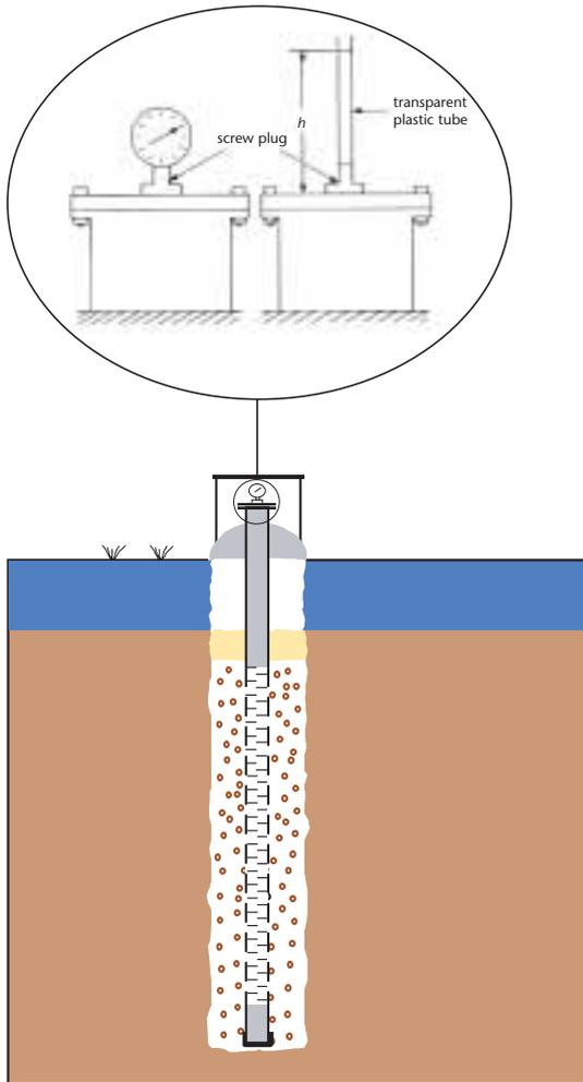
**Figure 7** | Monitoring set-up for artesian conditions
