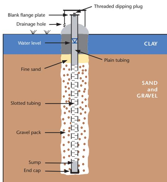
Figure 6 | Monitoring borehole for confined conditions
