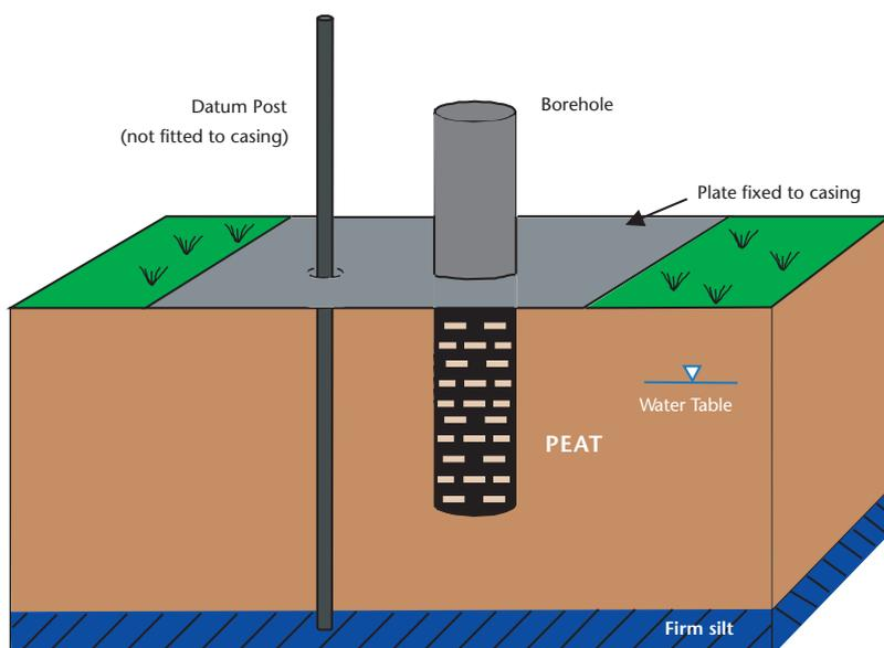
Figure 9 | Setting a borehole datum post
