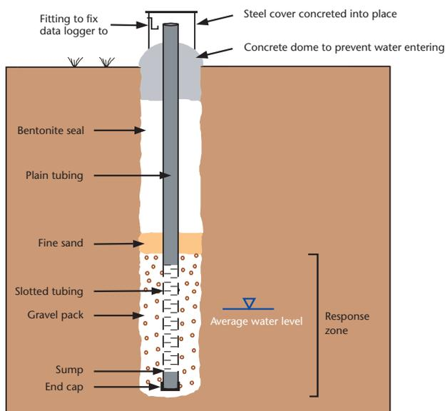
**Figure 5** | Monitoring borehole
