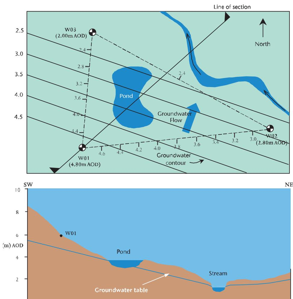
Figure 15 | Groundwater contours and cross-section
